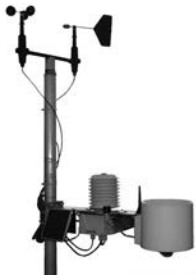
Internet weather station
